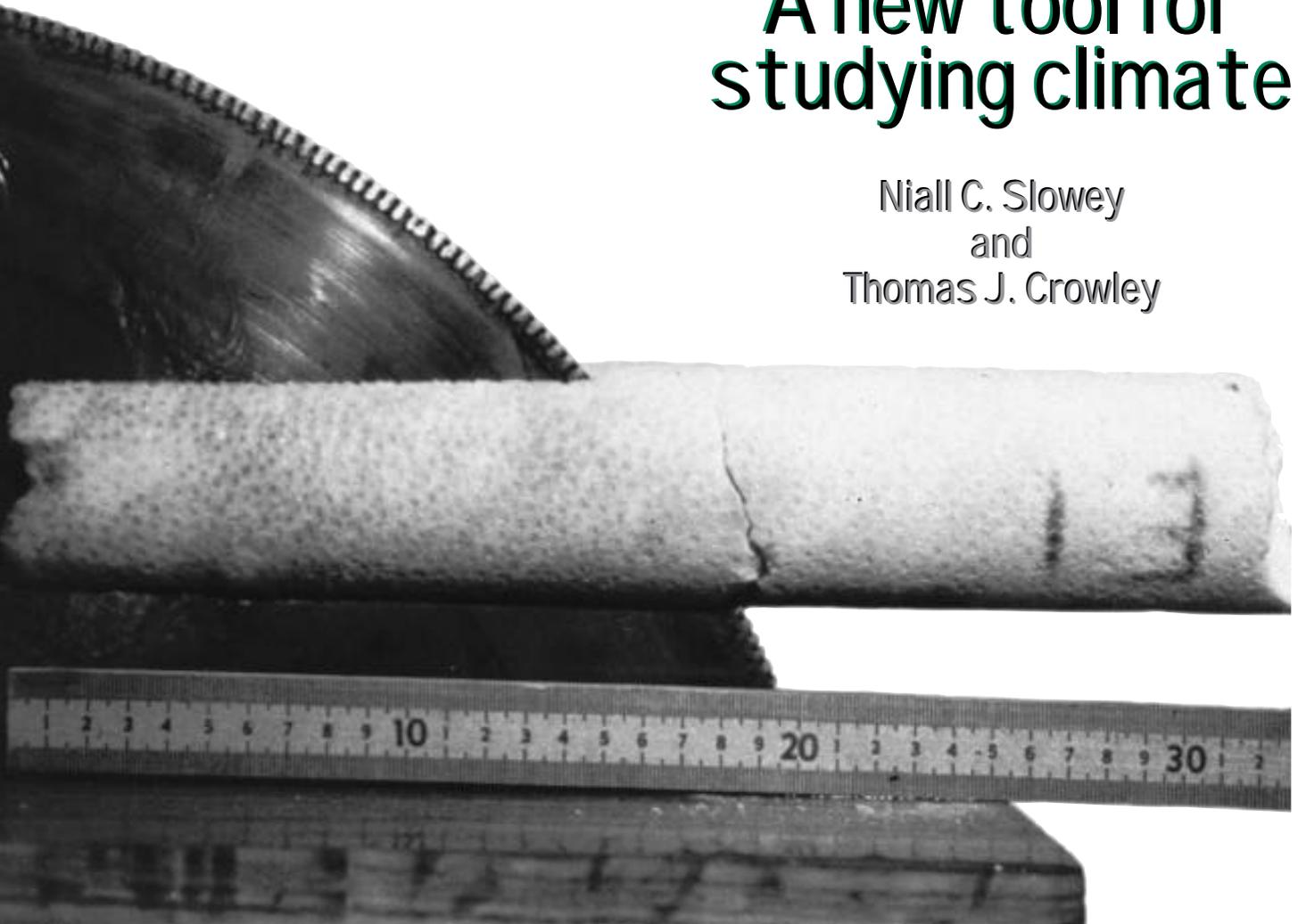
*A circular saw is used to cut slabs from a coral core. The slab will be x-rayed to reveal annual bands which preserve information about past climates. (Photo by Ken Deslarzes)*
