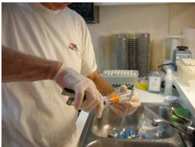
Figure 9 (left). Crushing the core with long-nosed pliers within the sample tube.
