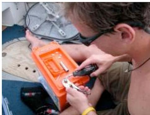
Figure 8 (right). Using Dremel tool to trim and section coral core.
