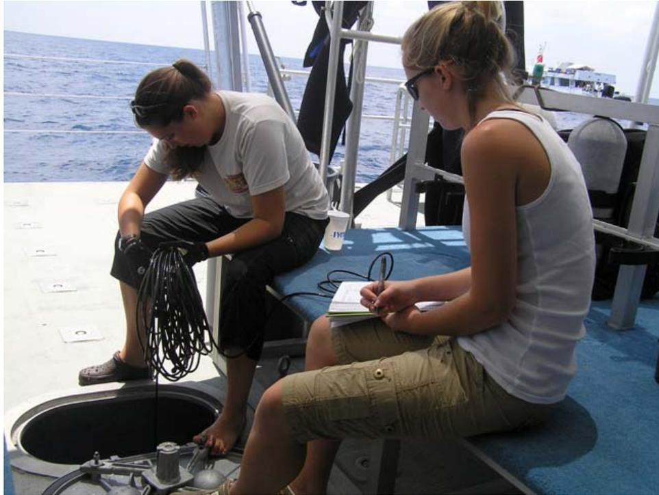
Fig. 3. Marissa Nuttall and Courtney deploy the YSI temperature/salinity probe through the moon pool, to collect profiles from surface down to 25m.
