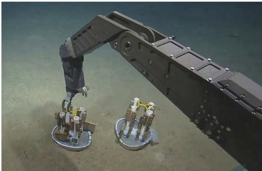
*The manipulator arm of the remotely operated vehicle deploys two sets of wood experiments that are assessing the biological colonization and rates of degradation of wood used to build 19th century ships.*
